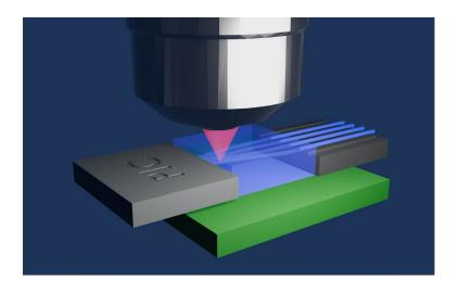
Illustration of Adaptive Optic Direct Laser Waveguide writing in glass connector block between
